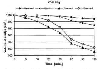
Fig. 5. Variation of settling characteristics during aerobic digestion  $-2^{rd}$  day.
