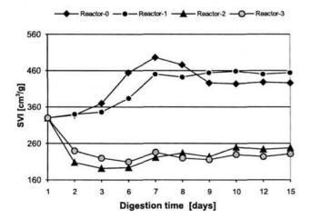
Fig. 4. SVI changes during aerobic digestion in the presence of H2O2 and Fenton's reagent.
