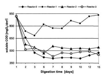
Fig. 1. COD changes for supernatants during aerobic digestion in the presence of  $H_2O_2$  and Fenton's reagent.
