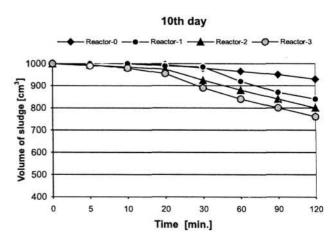
Fig. 7. Variation of settling characteristics during aerobic digestion -  $10^{\text{th}}$  day.
