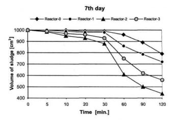
Fig. 6. Variation of settling characteristics during aerobic digestion  $-7^{\text{th}}$  day.
